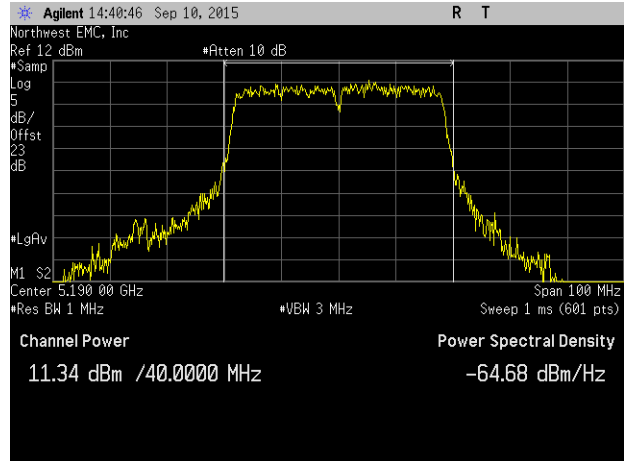
Chain C, 802.11(ac) VHT, MCS9 (256-QAM), 40 MHz, Low Channel 5190 MHz
