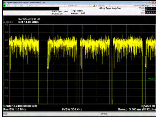
Chain C, 802.11(n) HT, MCS16, 20 MHz, High Channel 5240 MHz
