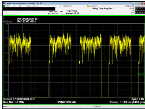
Chain A, 802.11(ac) VHT, MCS8 (256-QAM), 20 MHz, Low Channel 5180 MHz
