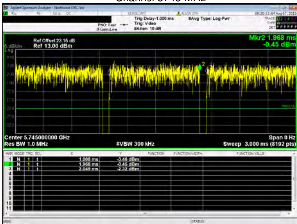
Chain B, 802.11(ac) VHT, MCS8 (256-QAM), 20 MHz, Low Channel 5745 MHz
