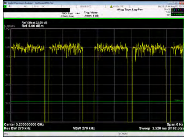
Chain C, 802.11(n) HT, MCS8, 40 MHz, High Channel 5230 MHz
