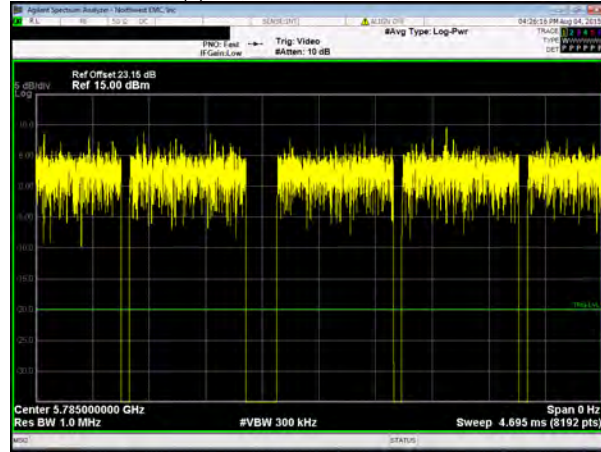
Chain C, 802.11(n) HT, MCS8, 20 MHz, Mid Channel 5785 MHz
