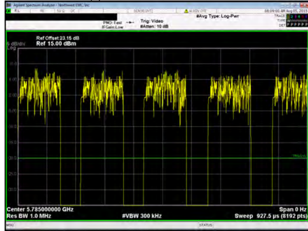
Chain C, 802.11(n) HT, MCS15, 20 MHz, Mid Channel 5785 MHz
