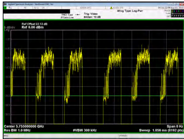
Chain C, 802.11(ac) VHT, MCS9 (256-QAM), 40 MHz, Low Channel 5755 MHz
