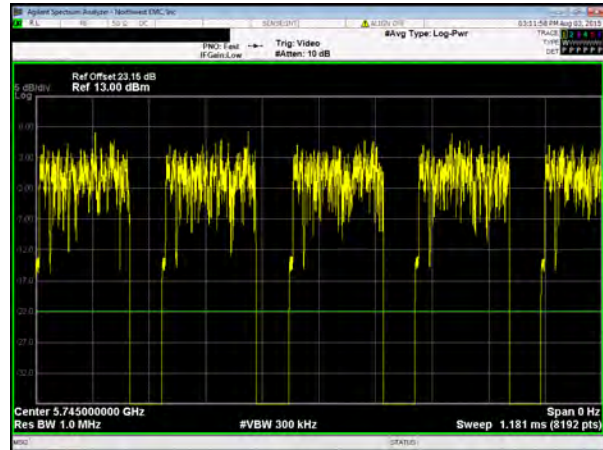
Chain C, 802.11(ac) VHT, MCS8 (256-QAM), 20 MHz, Low Channel 5745 MHz
