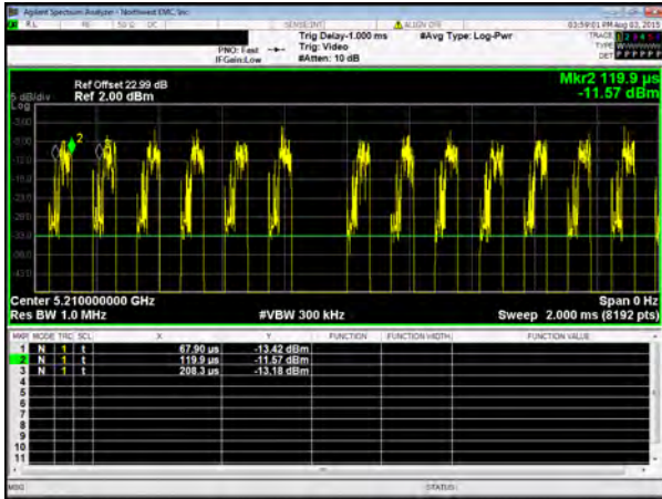
Chain C, 802.11(ac) VHT, MCS9 (256-QAM), 80 MHz, Low Channel 5210 MHz
