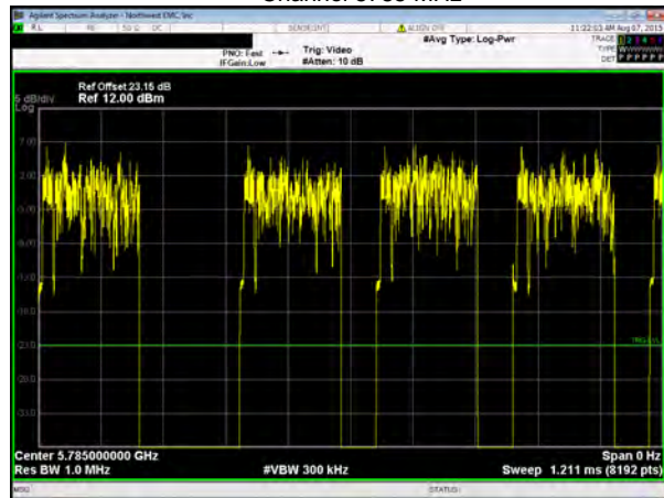
Chain C, 802.11(ac) VHT, MCS8 (256-QAM), 20 MHz, Mid Channel 5785 MHz
