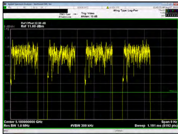
Chain C, 802.11(ac) VHT, MCS8 (256-QAM), 20 MHz, Low Channel 5180 MHz
