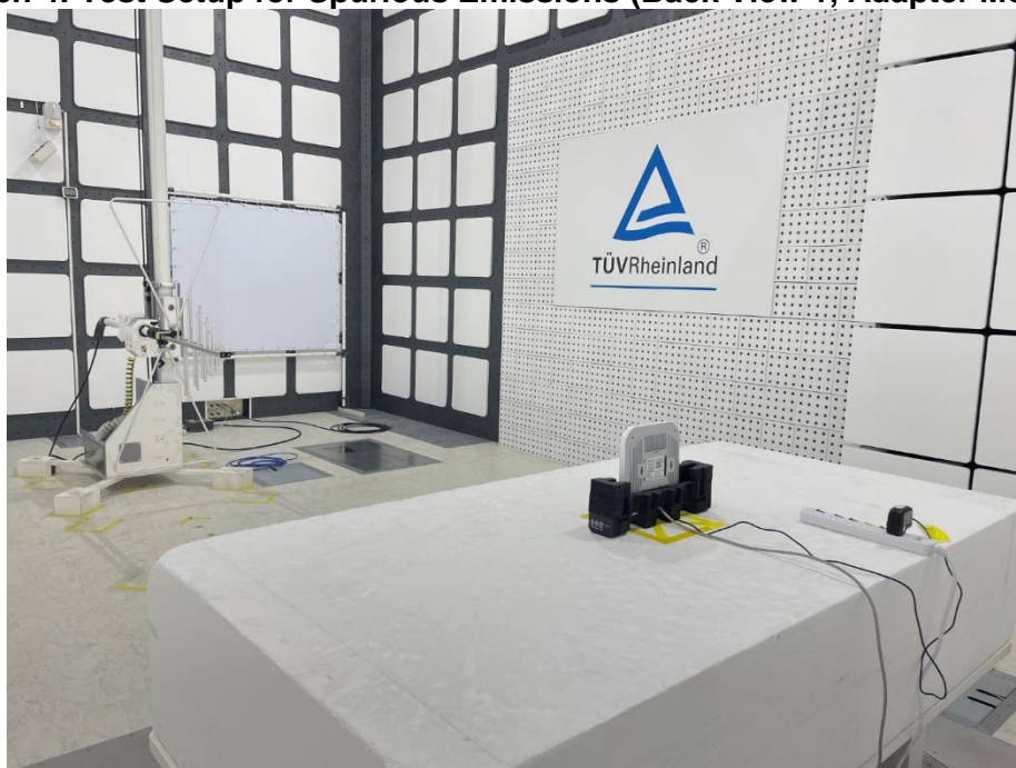
Photograph 4: Test Setup for Spurious Emissions (Back View 1, Adapter Mode)
