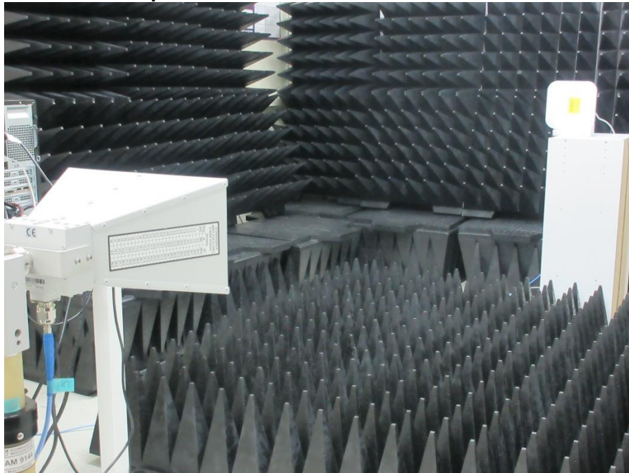
Photograph 17: Test Setup for DFS Mode
