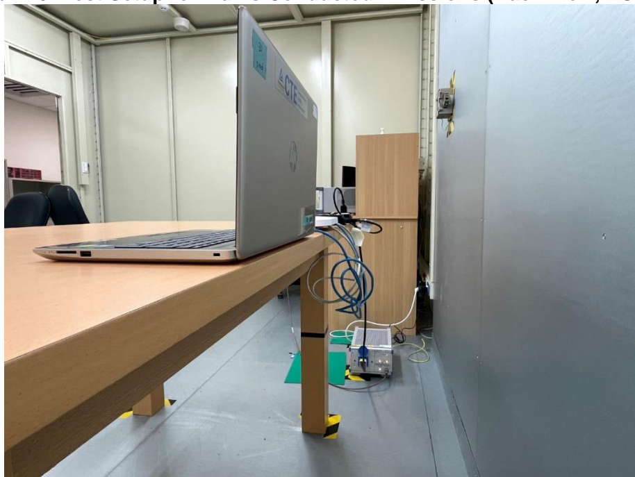
Photograph 16: Test Setup for Mains Conducted Emissions (Back View, POE Mode)
