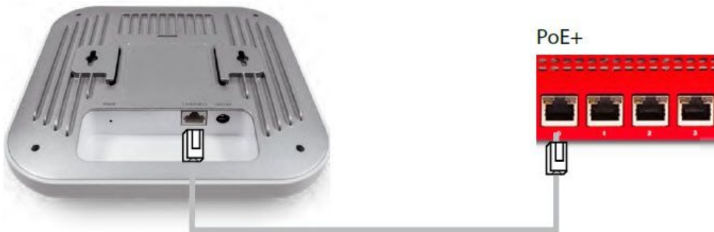
Access Point connected to switch with PoE+ power
