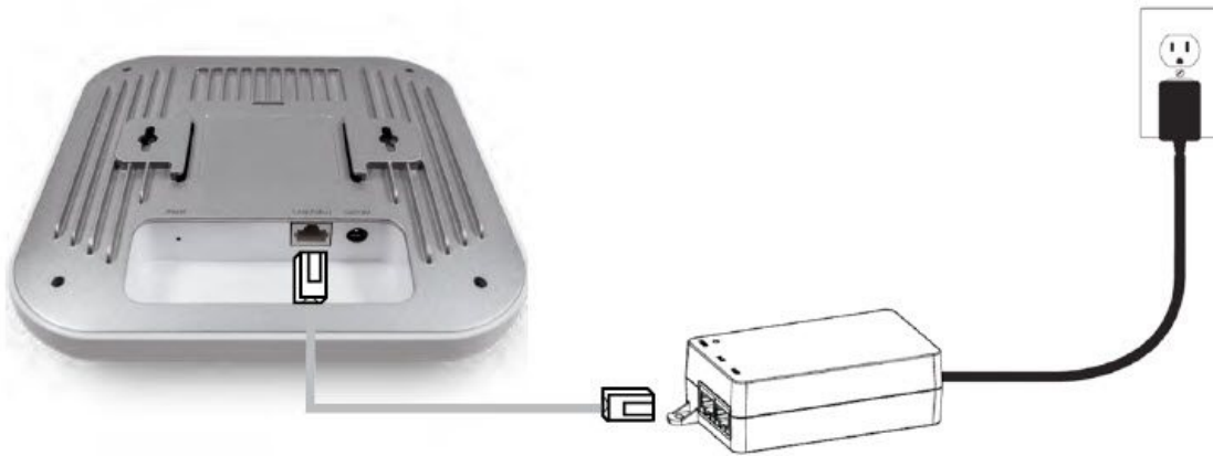
Access Point connected to PoE+ Injector
