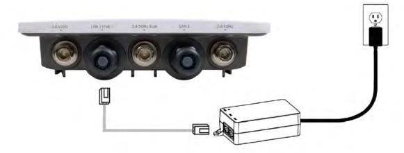
Access Point connected to PoE+ injector
