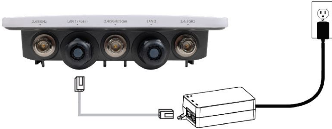
Access Point connected to PoE+ injector
