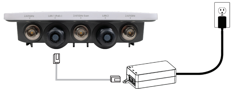
Access Point connected to PoE+ injector
