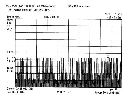
**NOTE:** (\*) Clarity of Time of Occupancy could not be satisfied using a 1 MHz resolution bandwidth. The resolution bandwidth was reduced in order to perform measurement.
