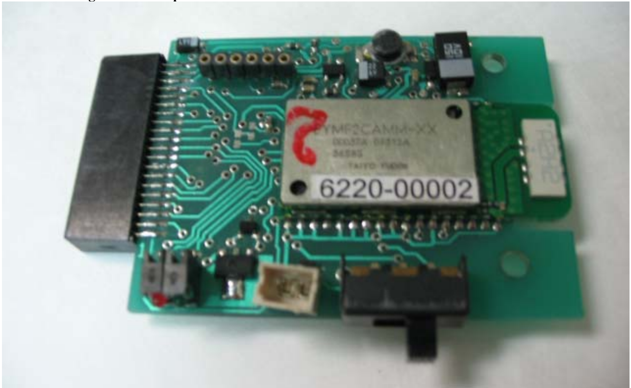
Blue Tooth Digital Board bottom view
