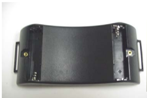
Head Unit Enclosure bottom outside
