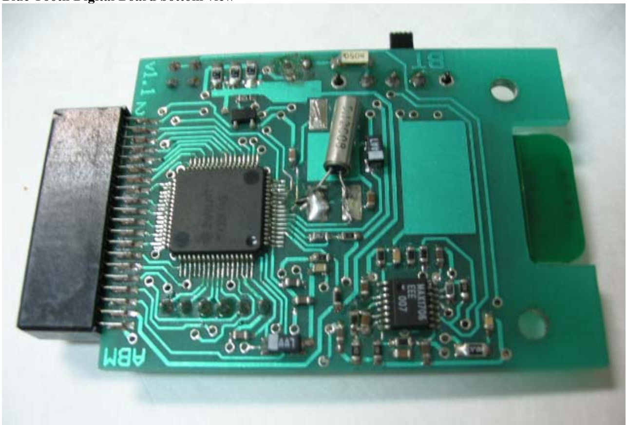
Blue Tooth Digital Board bottom view
