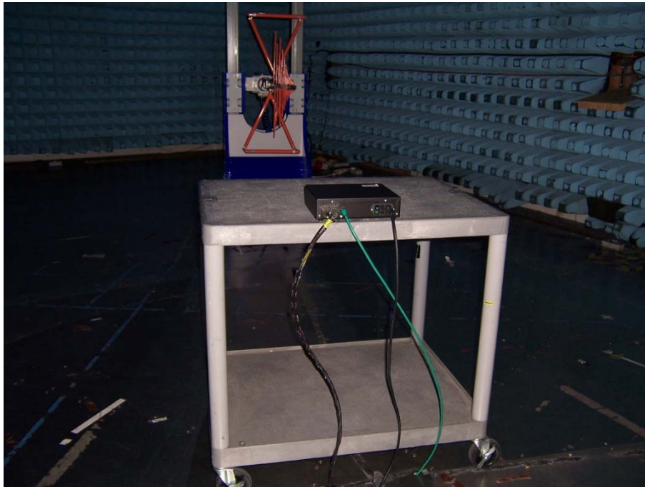
Figure 4 - Test Setup – Conducted Emissions
