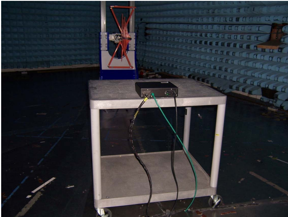
Figure 7 - Test Setup – Radiated Emissions Below 1 GHz
