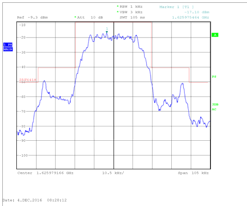
Figure 19 - 1625.979166 MHz - Emission Mask
