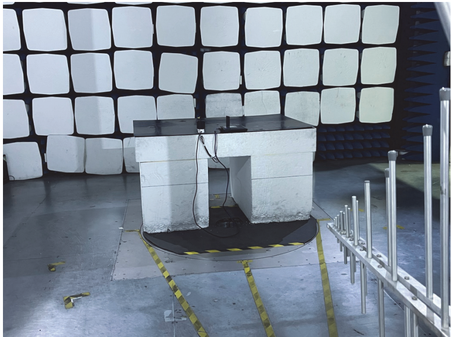
Radiation Emission Test View (30MHz to 1GHz)
