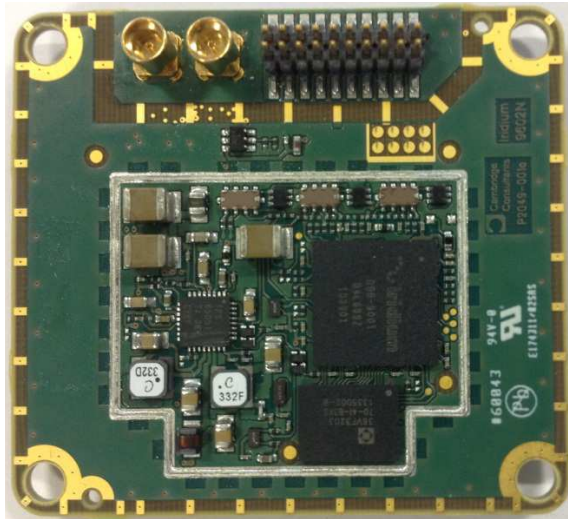
Figure 1 - Iridium 9602N top and bottom side views with bottom side screening can lid removed
