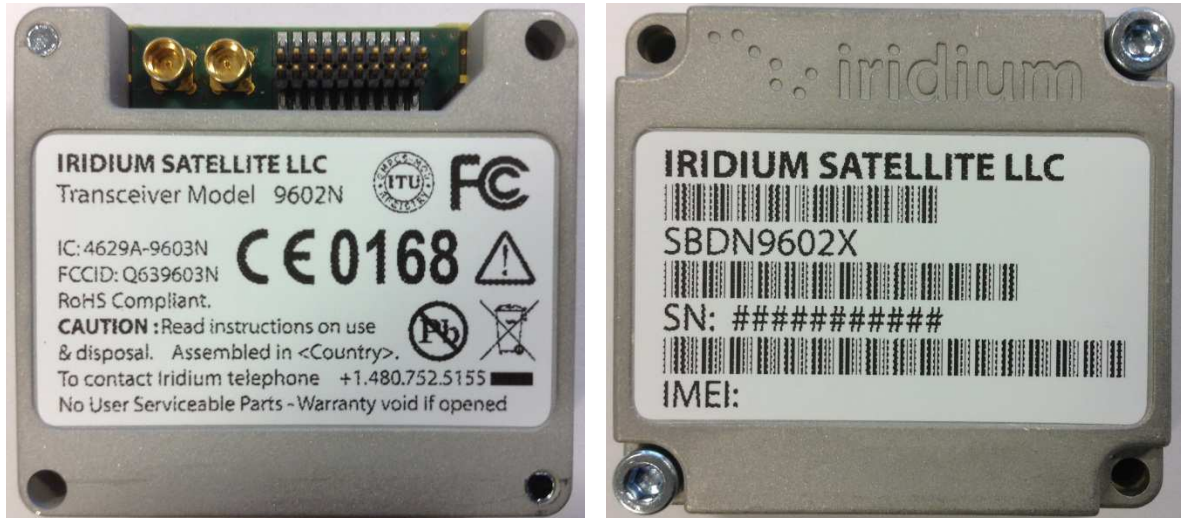
Figure 1 - Iridium 9602N top and bottom side external views
