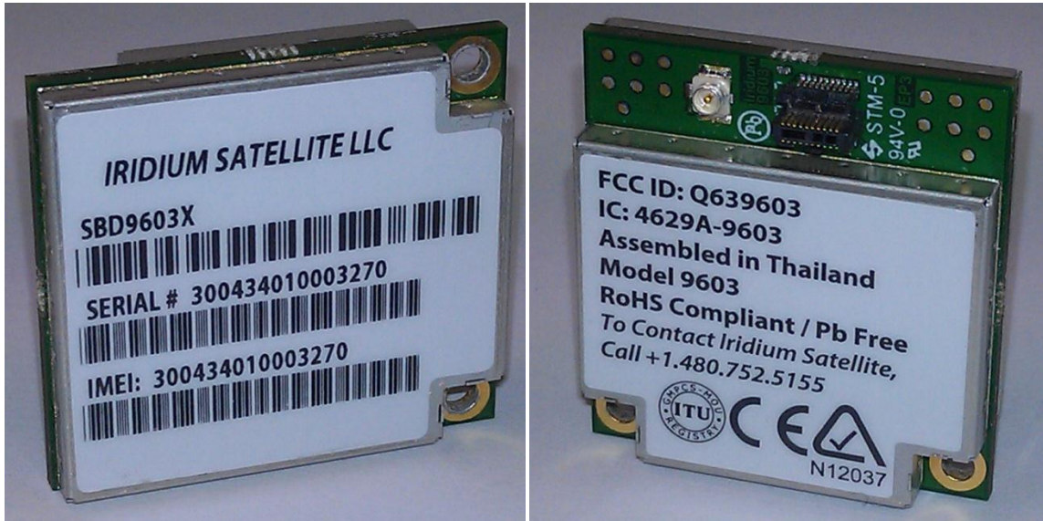
Figure 1. Iridium 9603 SBD Transceiver Front and Back Views
