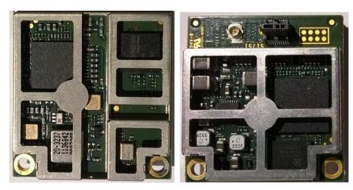
Figure 1 - Iridium 9603N top and bottom side views with casing removed
