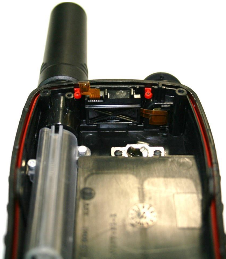
Figure 14 9575N – Back case inside showing location of Hands Free Speaker and Emergency Button flexi PCB
