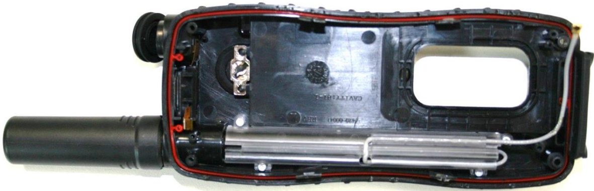
Figure 2 9575N – Back case inside showing antenna location
