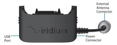
This adapter is to be used for charging the phone or connecting to a laptop via USB data cable when a wired, external antenna is used. This adapter provides a TNC connector that is compatible with the included 5' external antenna.
