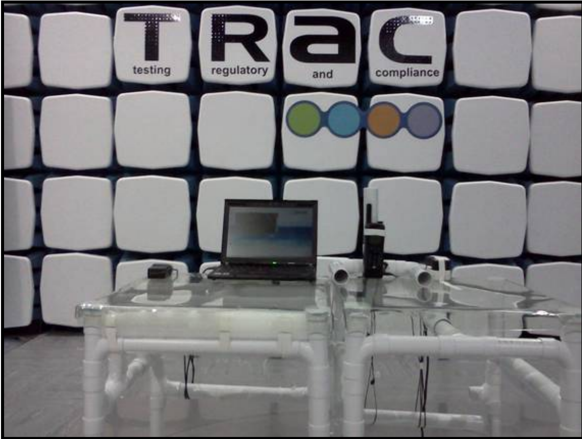
Radiated electric field emissions arrangement: Close up.
