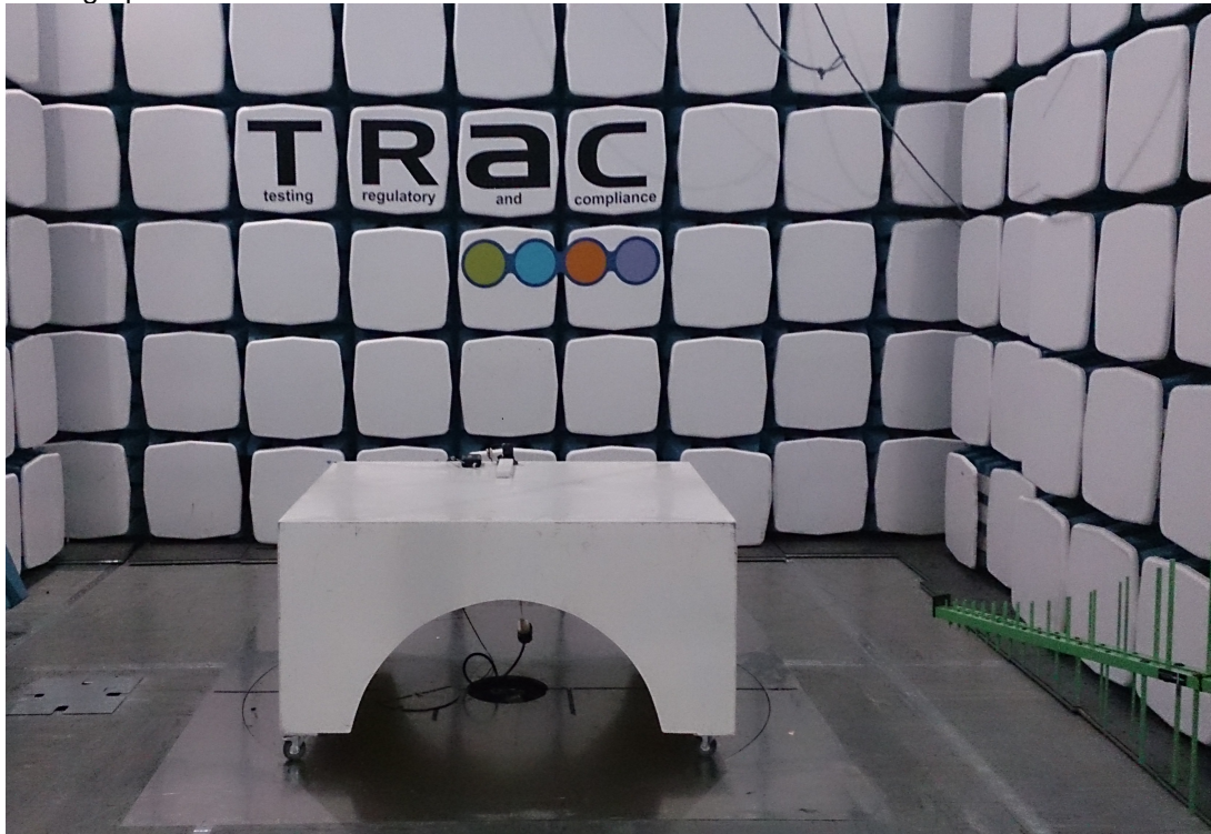
Photograph C2: RADIATED E-FIELD DISTURBANCE 30MHz – 1GHz
