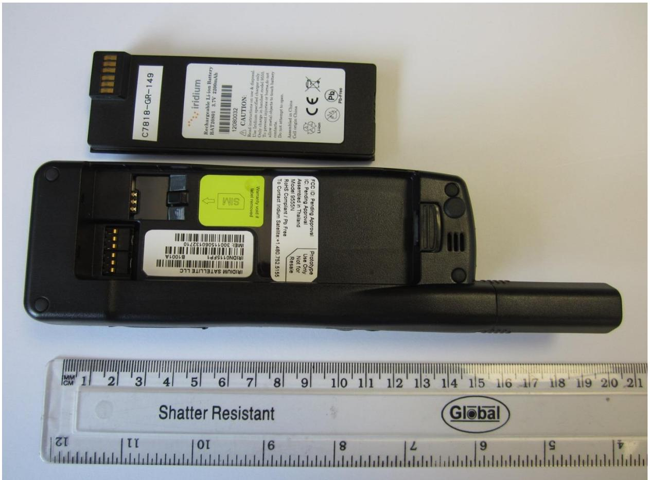
Rear View without battery (Regulatory and Manufacturing labels visible)
