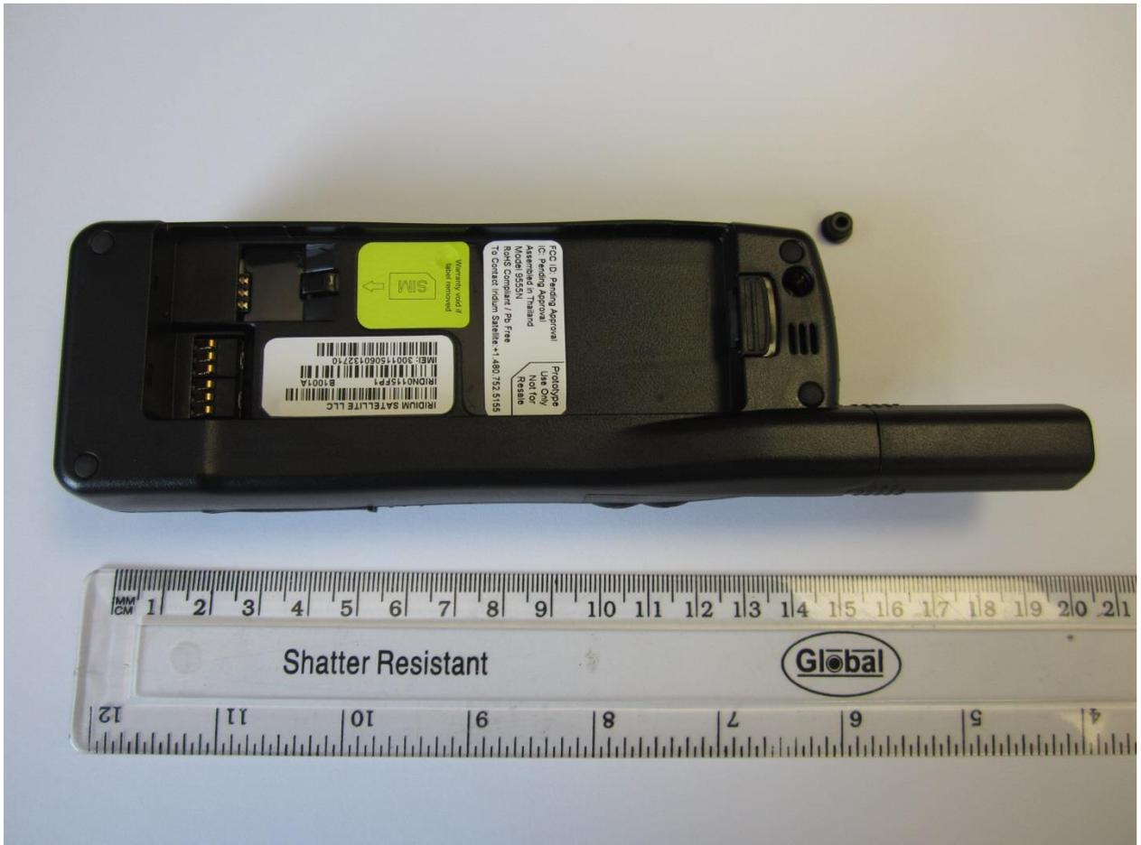
Rear View with External Antenna Port Plug Removed
