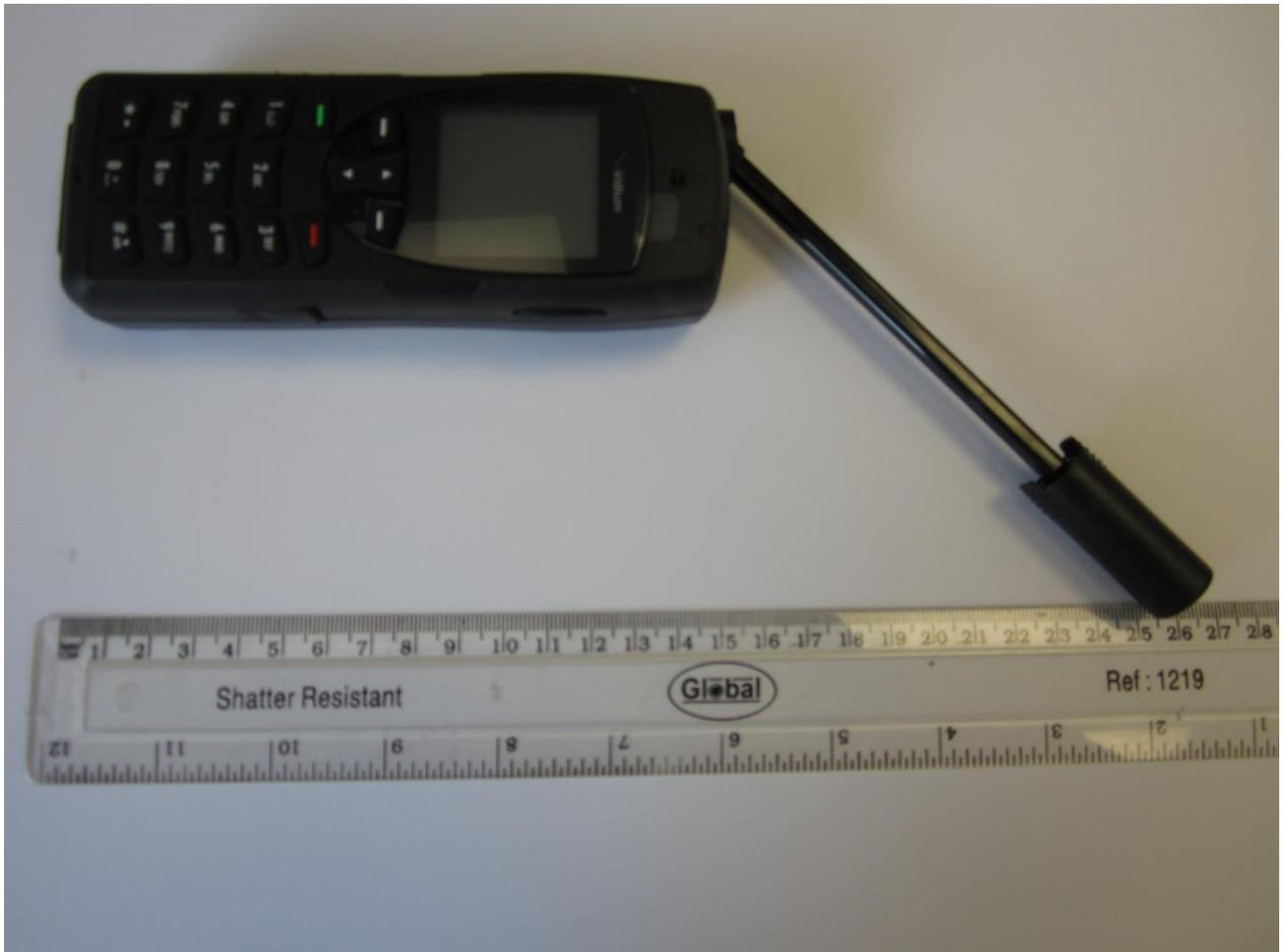
Front View with Antenna Deployed to the Side, It can go either way to be vertical in use
