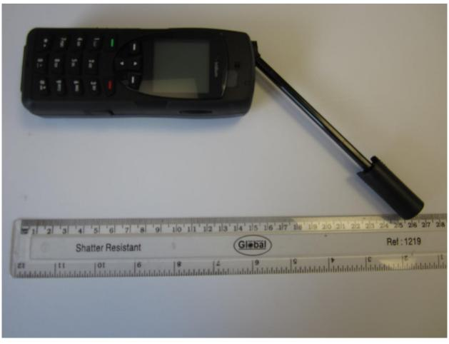
Front View with Antenna Deployed to the Side, It can go either way to be vertical in use
