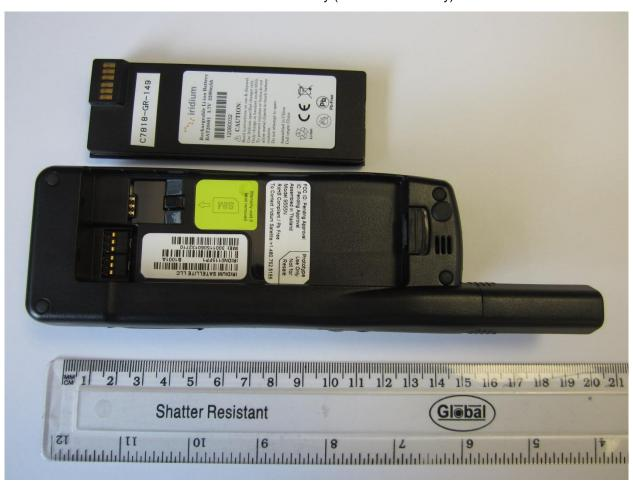
Rear View without battery (Regulatory and Manufacturing labels visible)
