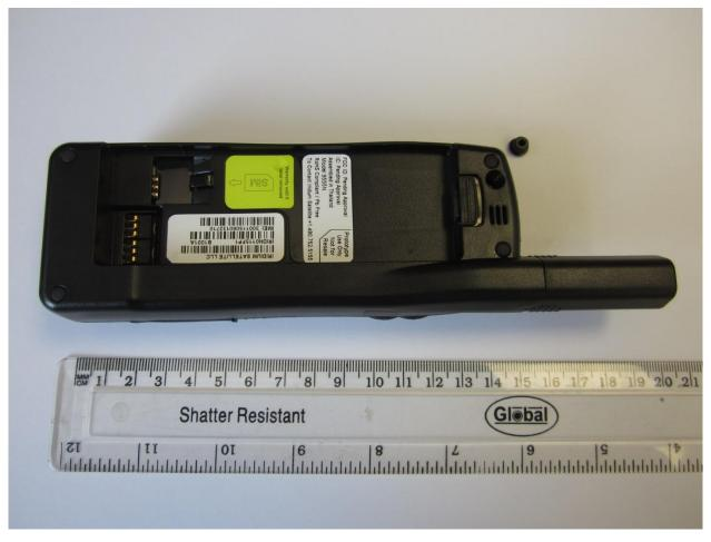
Rear View with External Antenna Port Plug Removed
