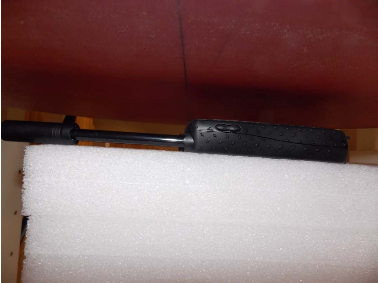
Test Position PTT Face Extended 25 mm Gap
