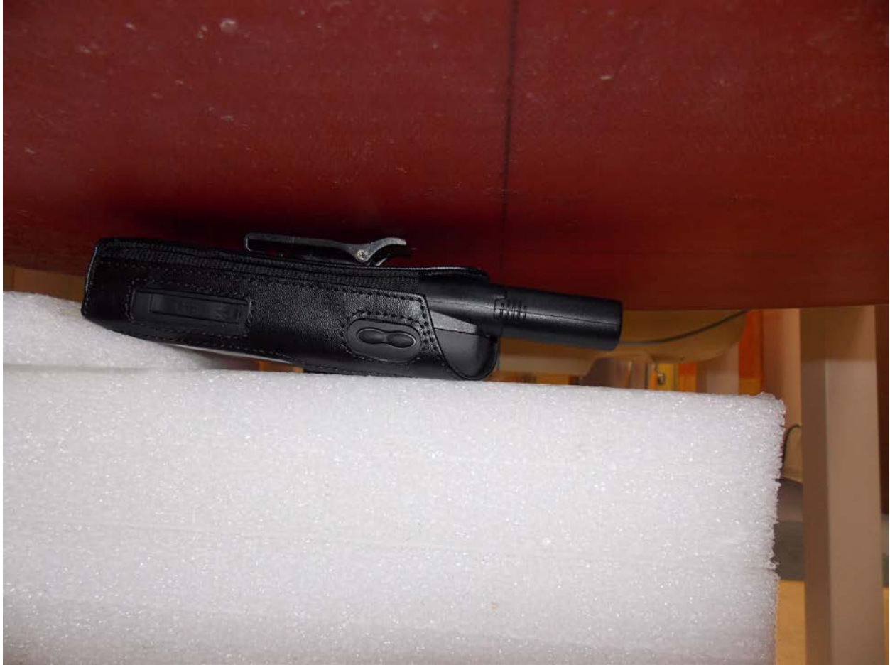
Test Position Body Retracted Touch 0 mm Gap
