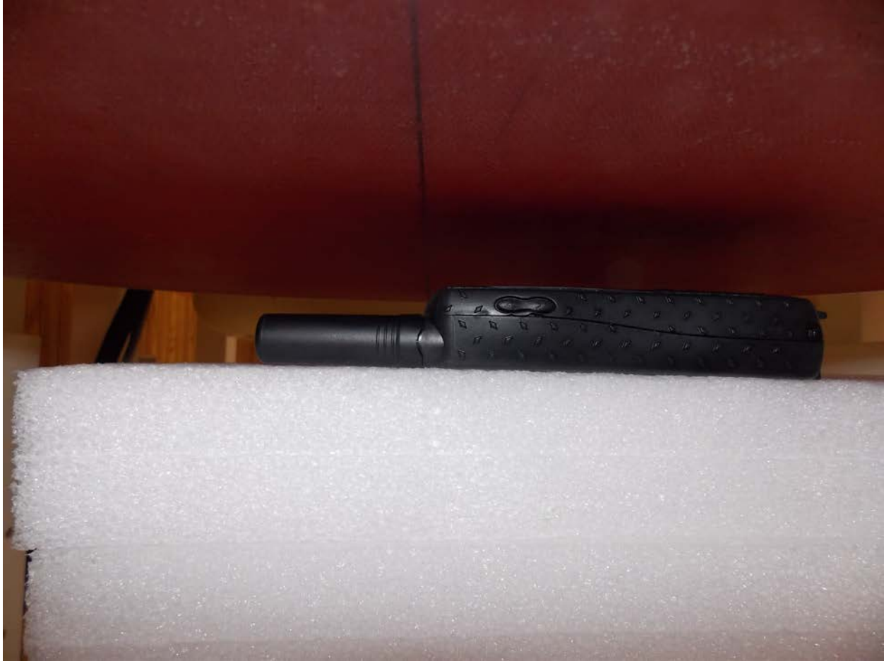
Test Position PTT Face Retracted 25 mm Gap
