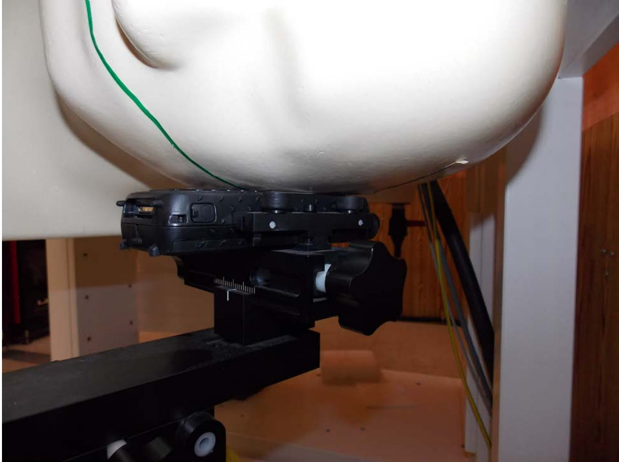
Test Position Left Head Retracted Touch 0 mm Gap
