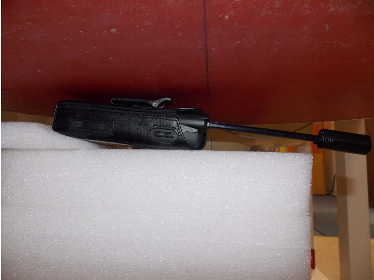
Test Position Body Extended Touch 0 mm Gap
