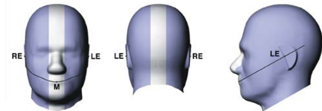
Figure 3.2 Front, back and side view of SAM
