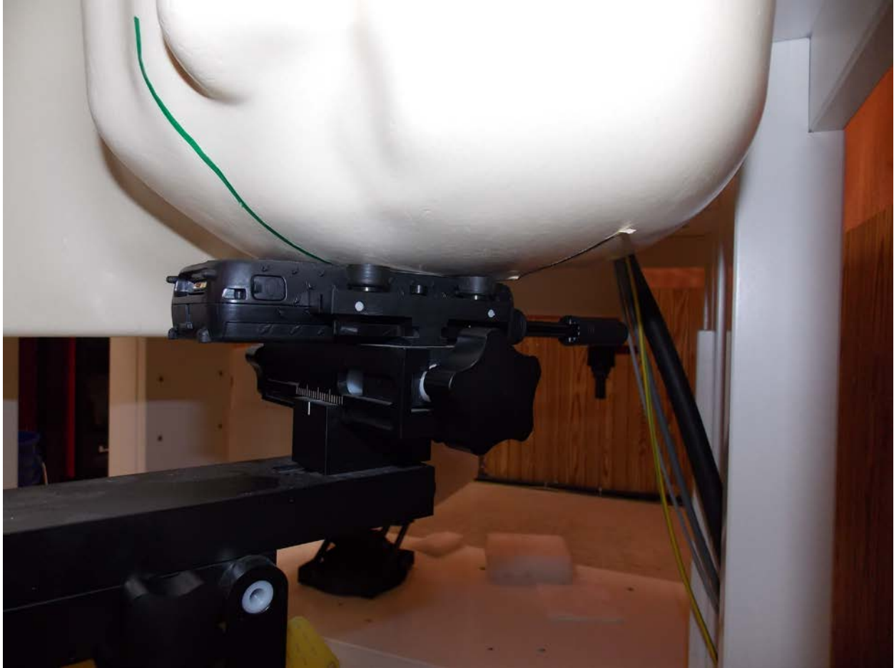
Test Position Left Head Extended Touch 0 mm Gap
