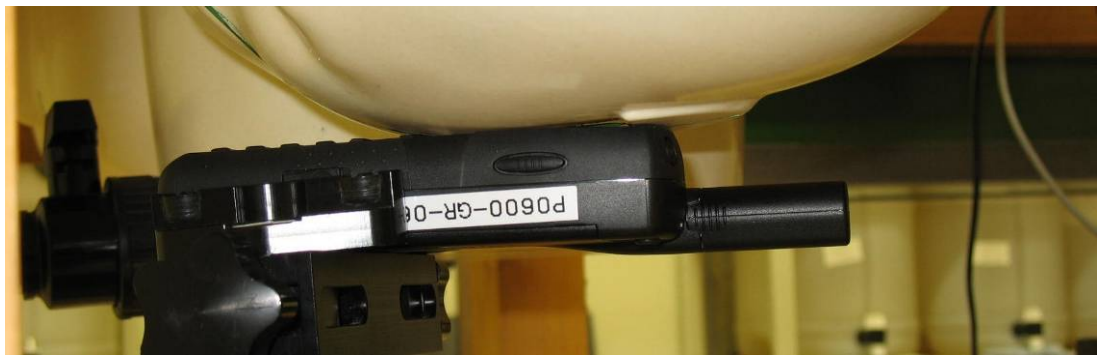
Touch Right Position - Antenna Retracted (IN)
