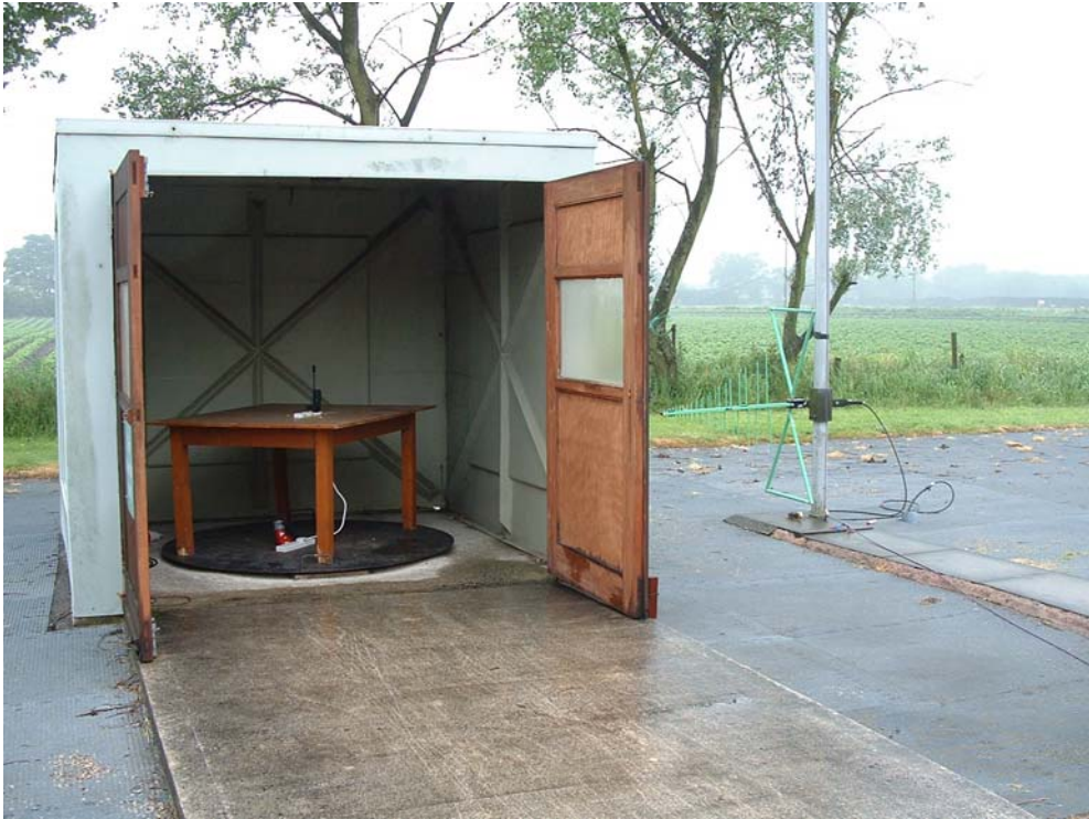
EUT On open Area Test Site
