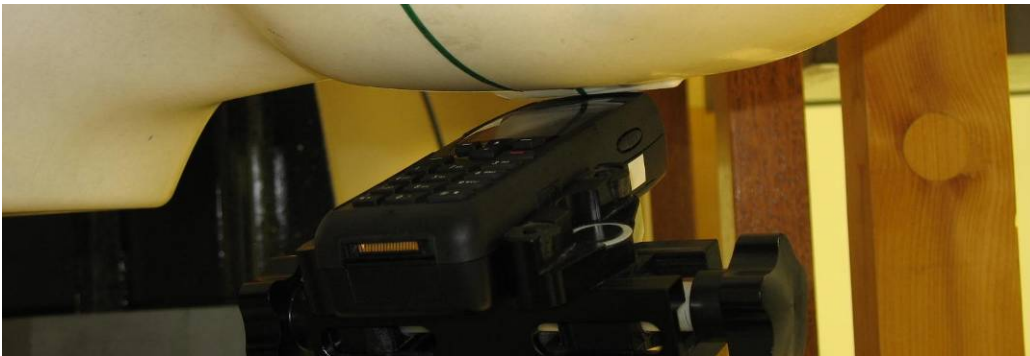
Tilted Left Position - Antenna Retracted (IN)
