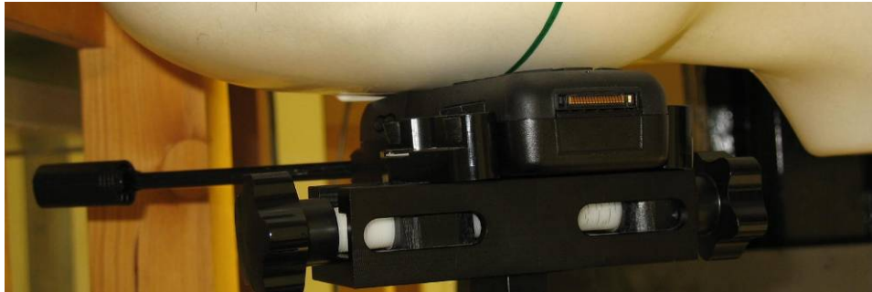
Touch Right Position - Antenna Extended (Out)
