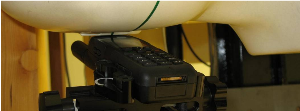
Tilted Right Position - Antenna Retracted (IN)
