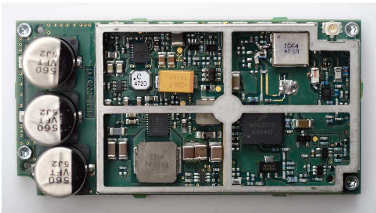
Figure 2 – 9523N rev B/V1 – Top View with screening can lid removed
