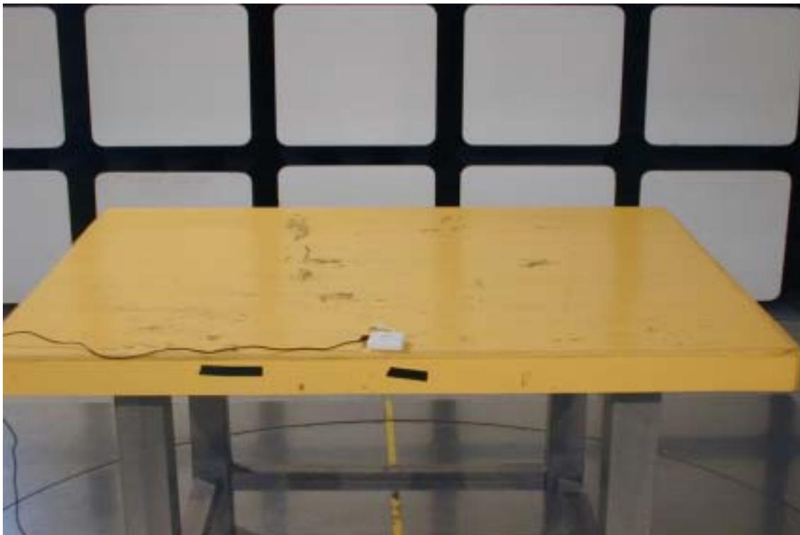
**Radiated Emission Set up Photo (Audio-In Mode)**
