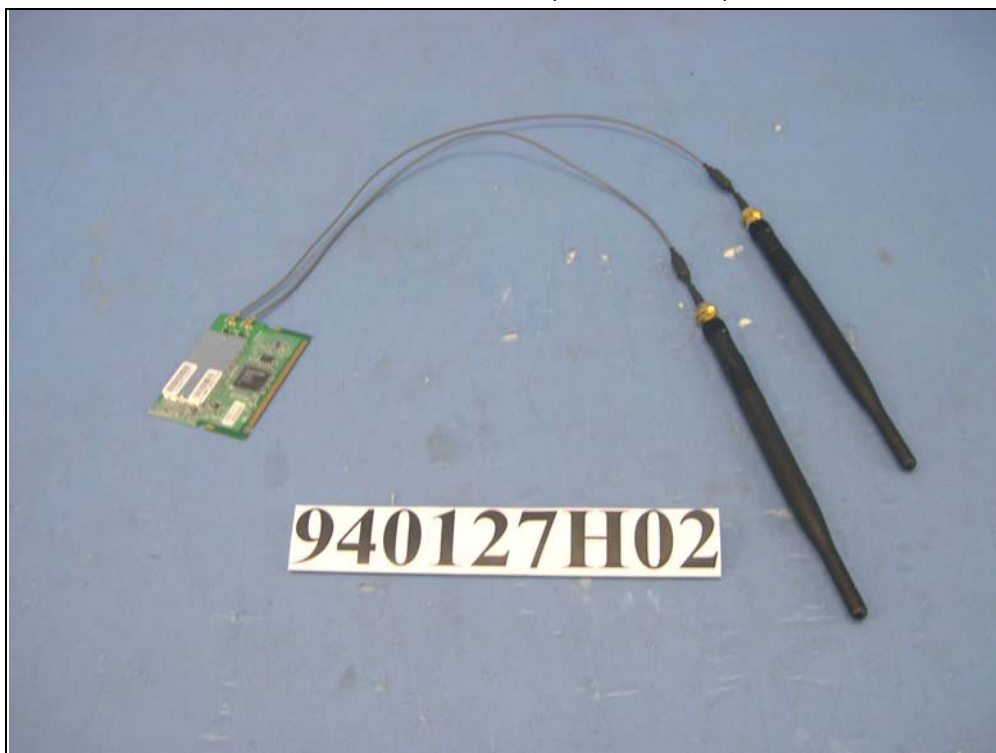
EUT with Antenna 5 (Cable: 32cm)
