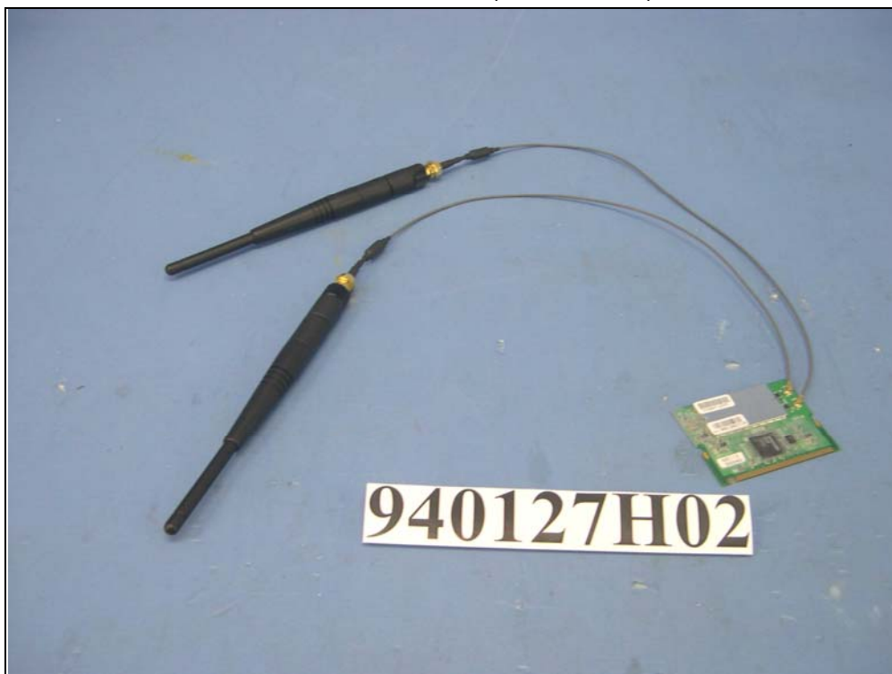
EUT with Antenna 6 (Cable: 32cm)
