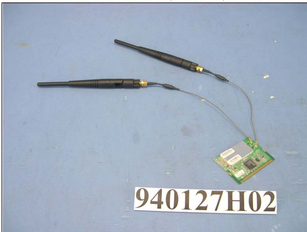
EUT with Antenna 6 (Cable: 16cm)
