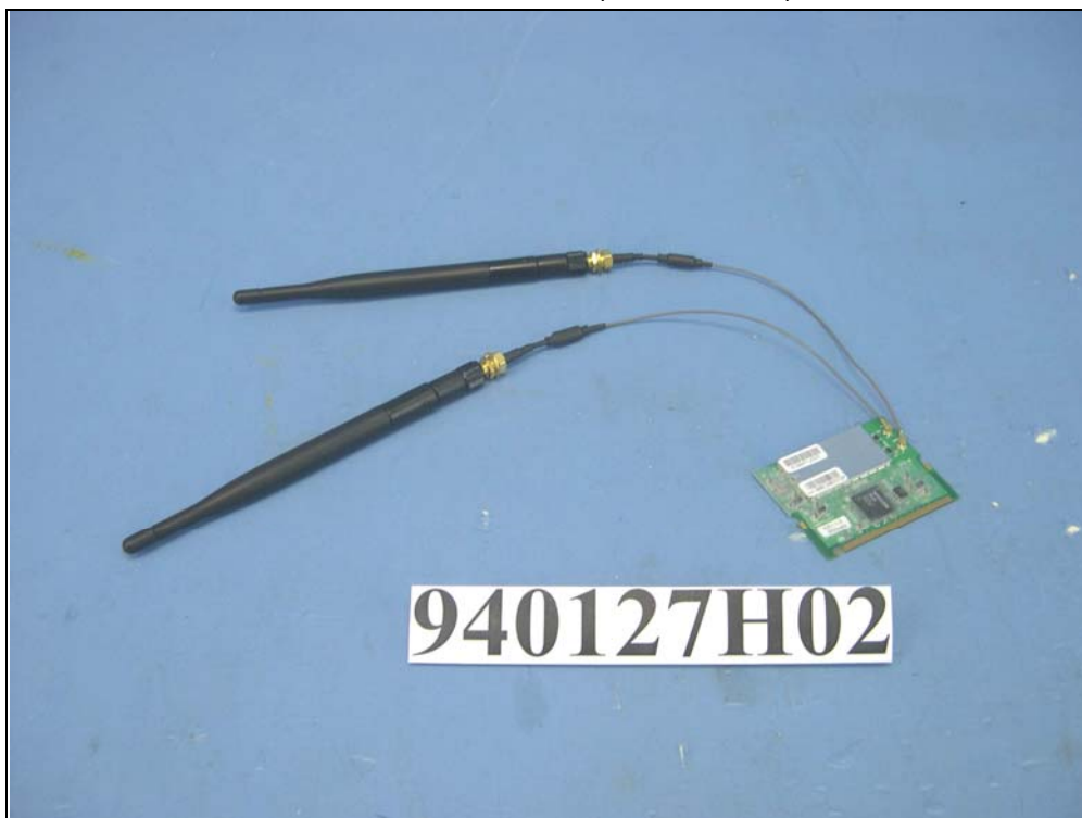
EUT with Antenna 5 (Cable: 16cm)
