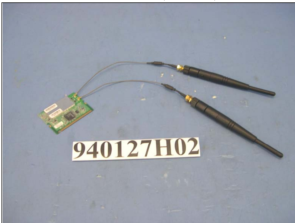
EUT with Antenna 4 (Cable: 16cm)
