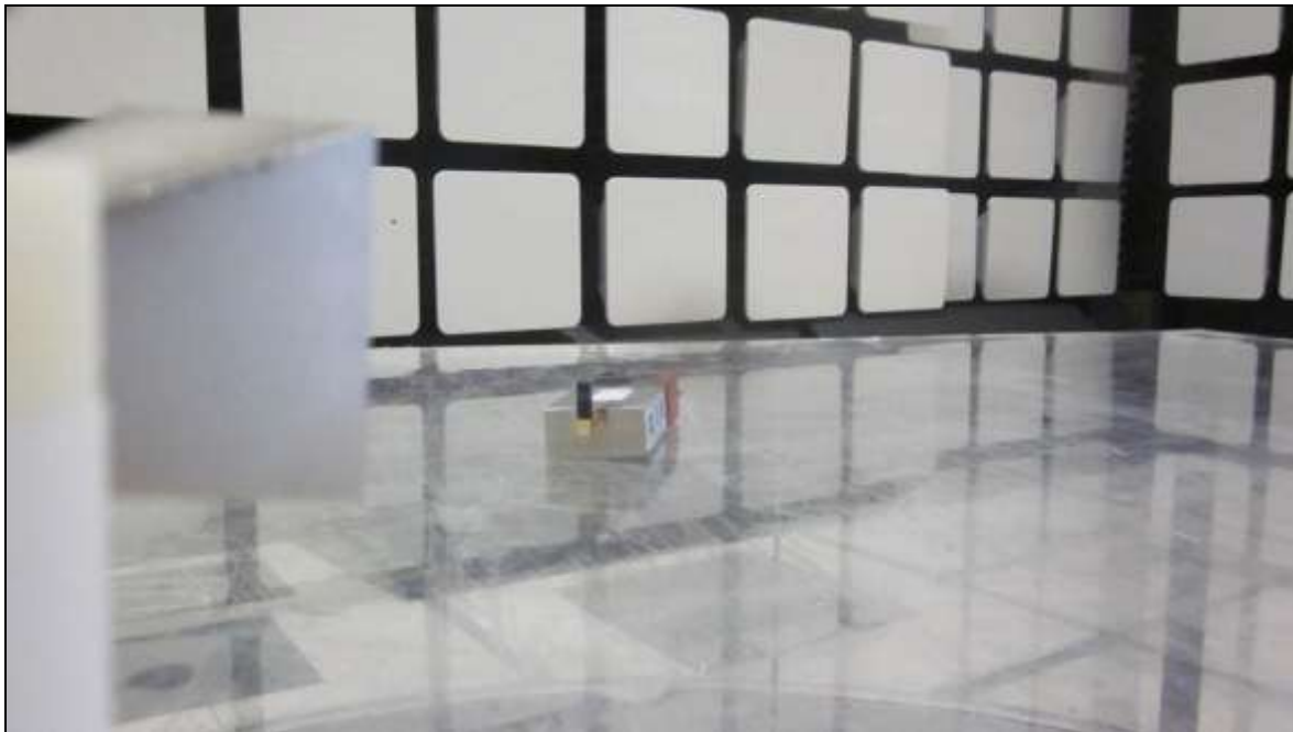
Photograph 4. Radiated Spurious Emissions, Test Setup, 18 GHz – 26 GHz
