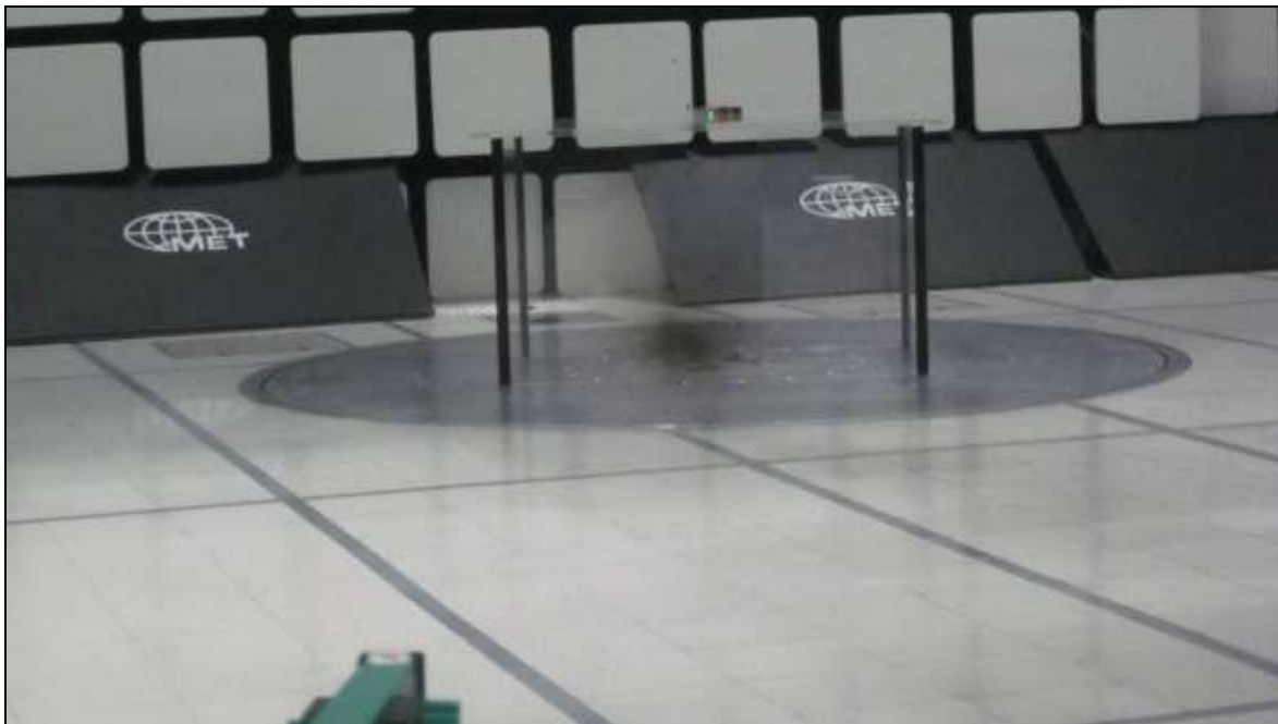
Photograph 2. Radiated Spurious Emissions, Test Setup, Below 1 GHz
