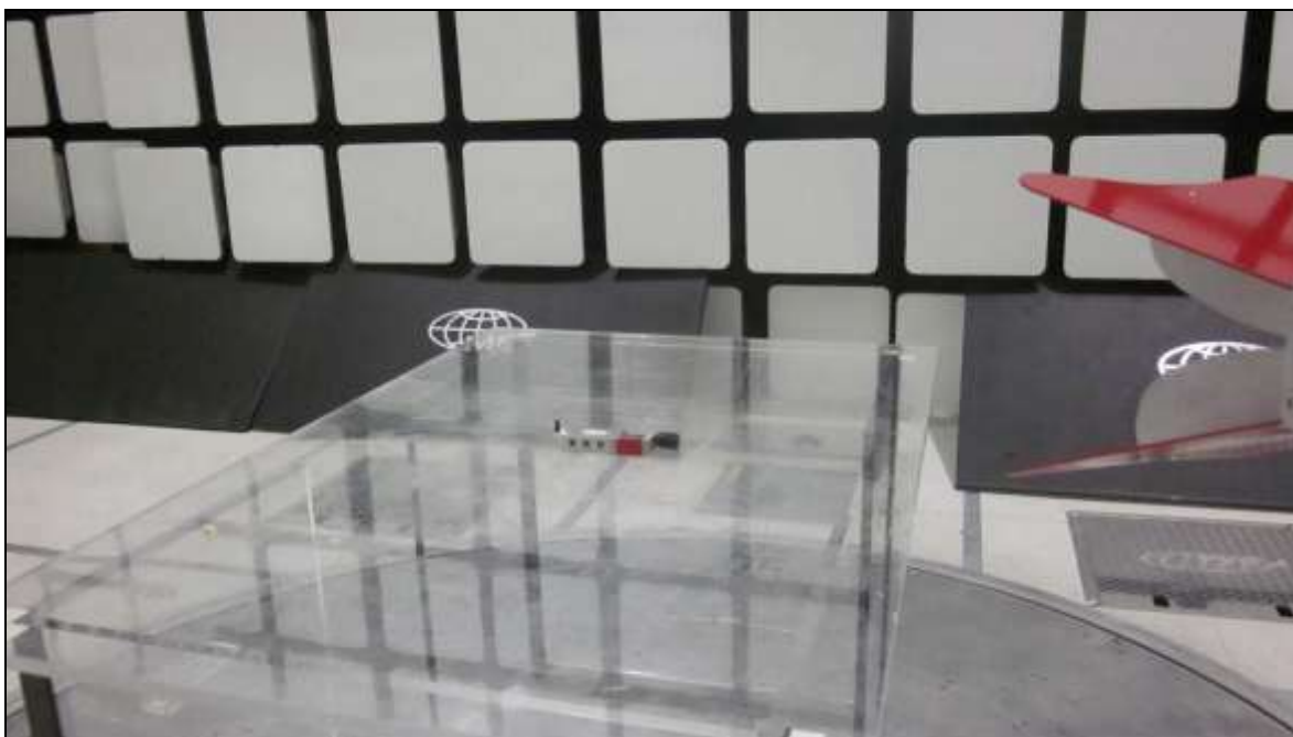
Photograph 3. Radiated Spurious Emissions, Test Setup, 1 GHz – 18 GHz
