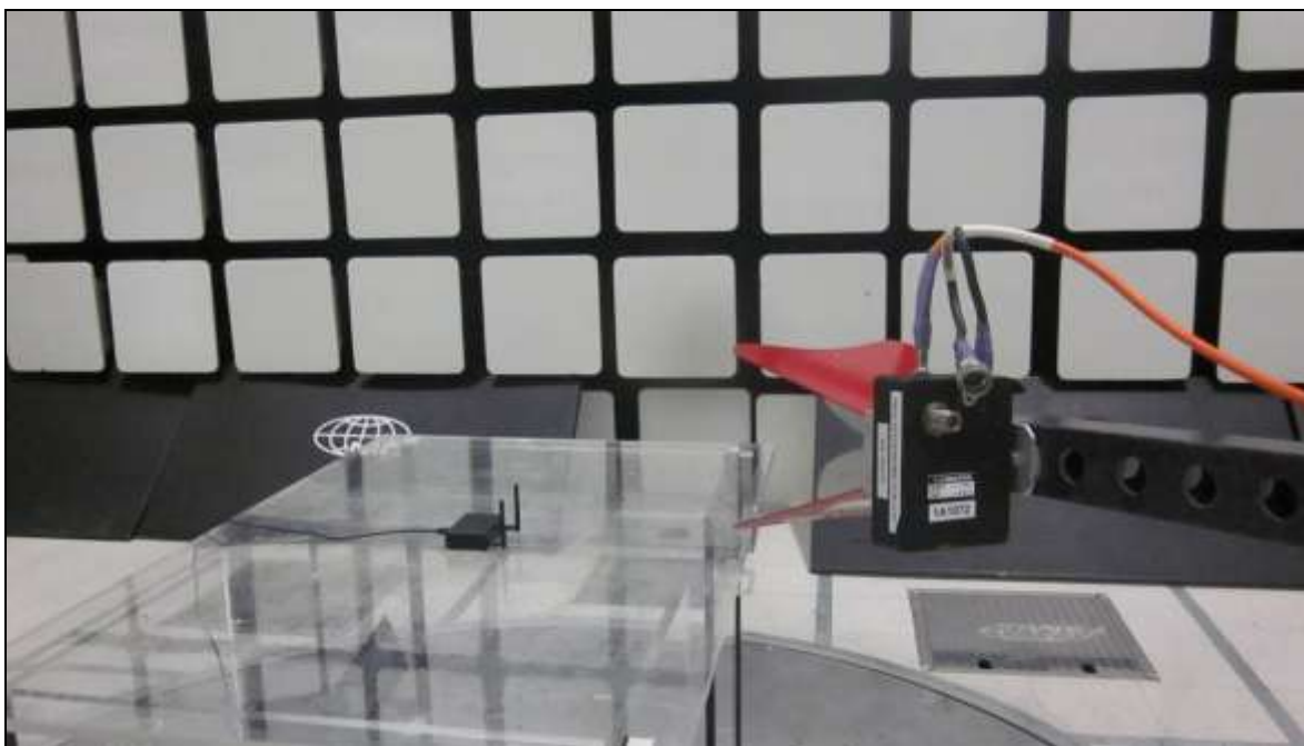
Photograph 3. Radiated Spurious Emissions, Test Setup, 1 GHz – 18 GHz
