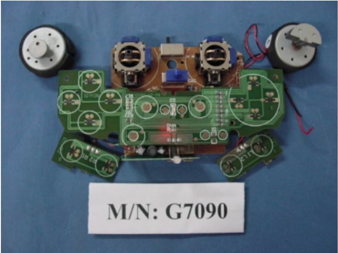
Figure 14 Main Board, Component Side
