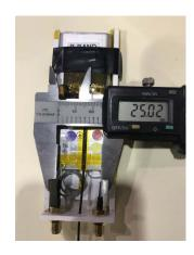
Peak SAR location distance measured at feed points of antenna pairs: r1 = 25.02mm r2 = 44.59mm
