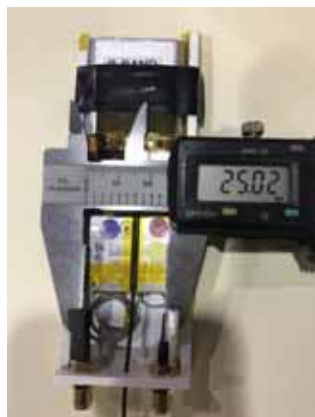
Peak SAR location distance measured at feed points of antenna pairs: r1 = 25.02mm r2 = 44.59mm
