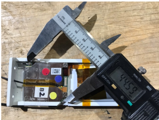
Peak SAR location distance measured at feed points of antenna pairs: r1 = 25.02mm r2 = 44.59mm
