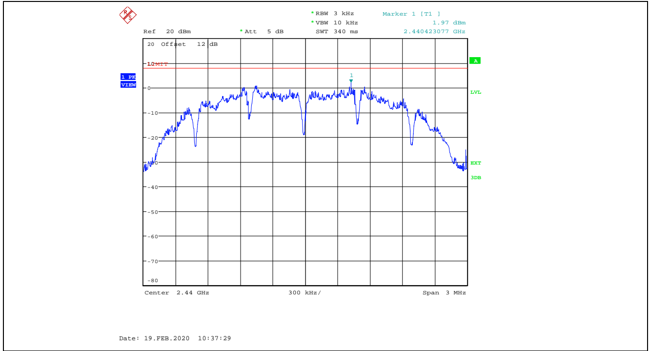
Plot 5.5.5.2. Power Spectral Density, Channel 18, 2440 MHz, MSK modulation, Power Setting 22
