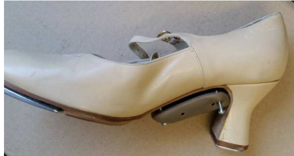
Figure 5 - Transmitter Pod attached to Shoe
