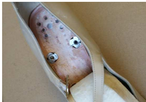
Figure 4 - T-Nuts installed into sole
