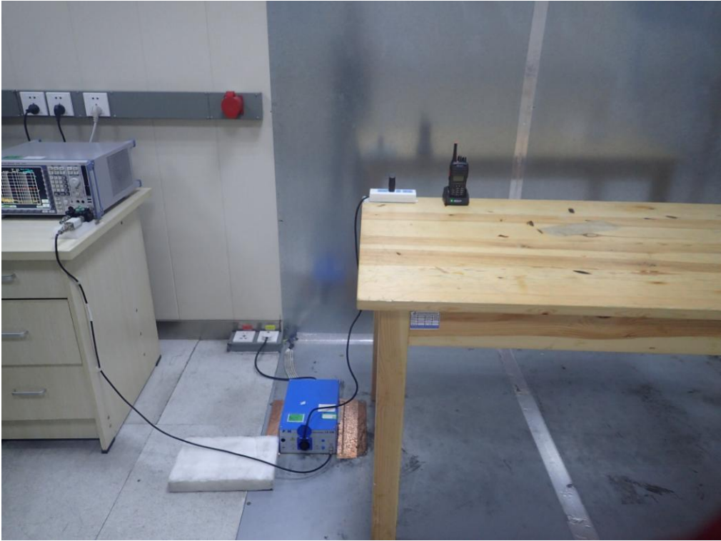
FCC RADIATED EMISSION TEST SETUP
