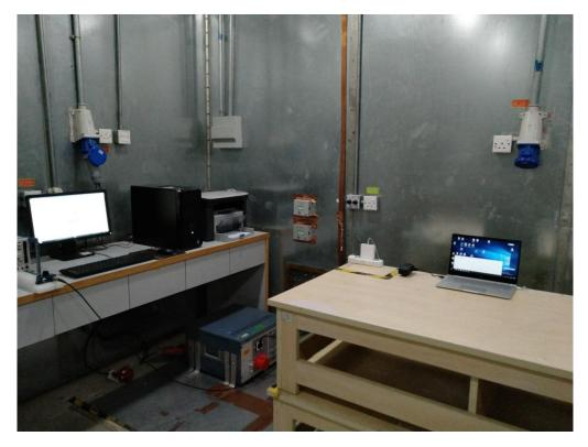
FCC RADIATED EMISSION TEST SETUP
