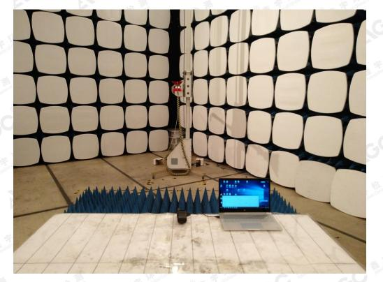
FCC RADIATED EMISSION TEST SETUP
