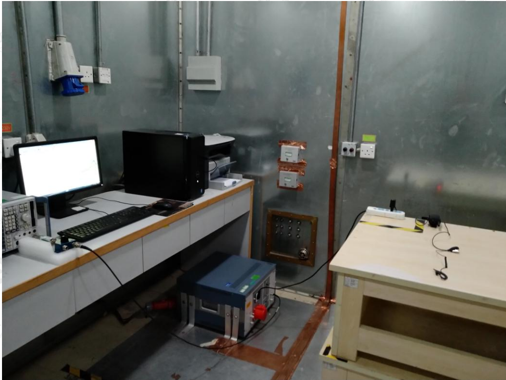
RADIATED EMISSION TEST SETUP
