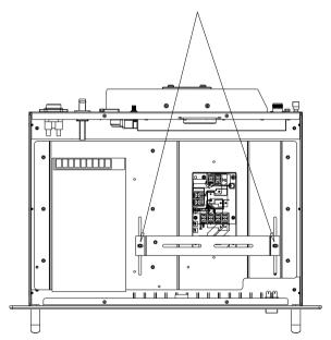
(4) Fixed the duplexer tail screws to the duplexer bracket. Push the duplexer to the end three duplexer connection holes until the duplexer is locked. Then fasten the duplexer bracket and install screw. Refer to following figure.
