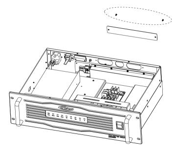
(3) Slightly loosen the two screws of fixed duplexer bracket on installed clapboard to the bracket, and do not too loosen. Refer to following figure.
