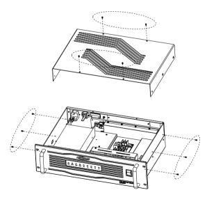
(2) Take off the two screws of duplexer baffle, remove the duplexer.
