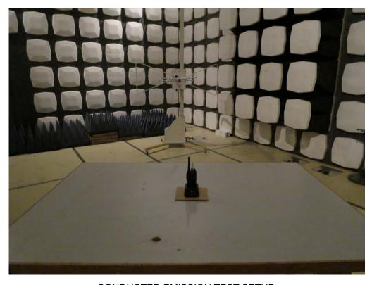
CONDUCTED EMISSION TEST SETUP
