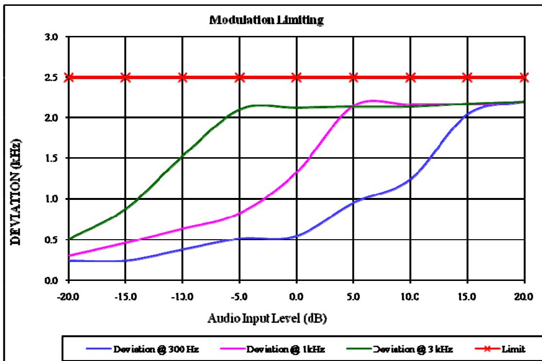
Note: the maximum frequency deviation is 2.2 kHz, which was declared by the manufactory.
