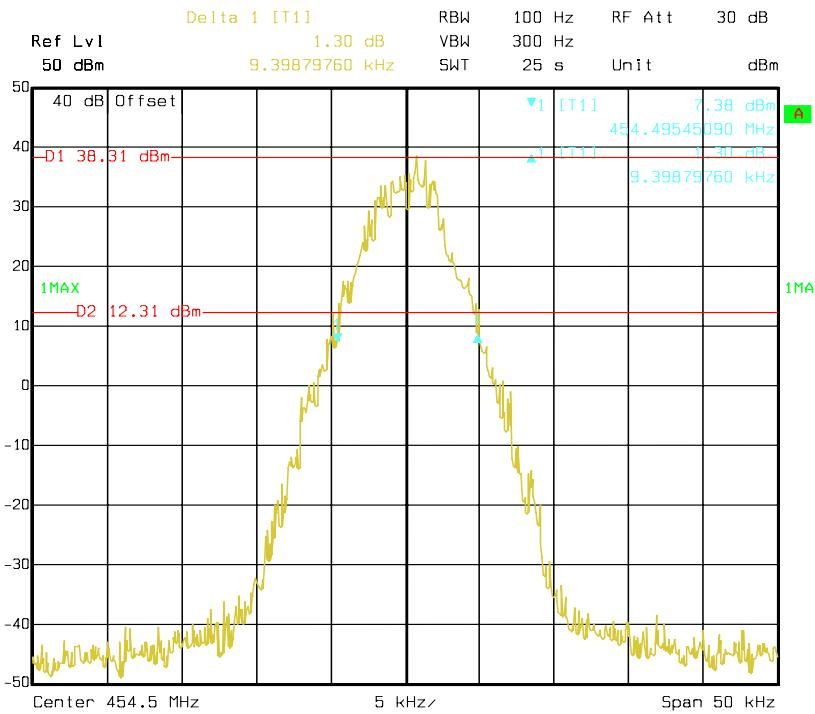
**Occupied Bandwidth -4FSK, 458MHz, Highest Power Level**
