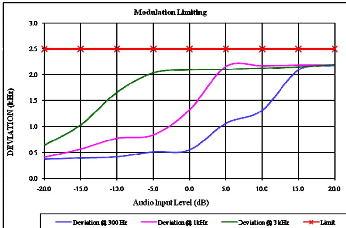
Note: the maximum frequency deviation is 2.2 kHz, which was declared by the manufacturer.
