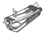
1. Put the two stop blocks at the top of the battery into the two slots at the back of the terminal.
