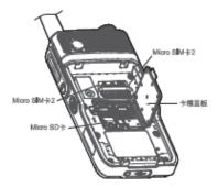
Open the card socket cover, and insert a micro SIM card and a micro-SD card as instructed on the cover.
