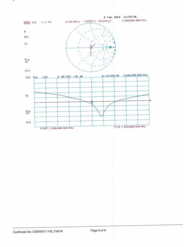
Impedance Measurement Plot for Head TSL
