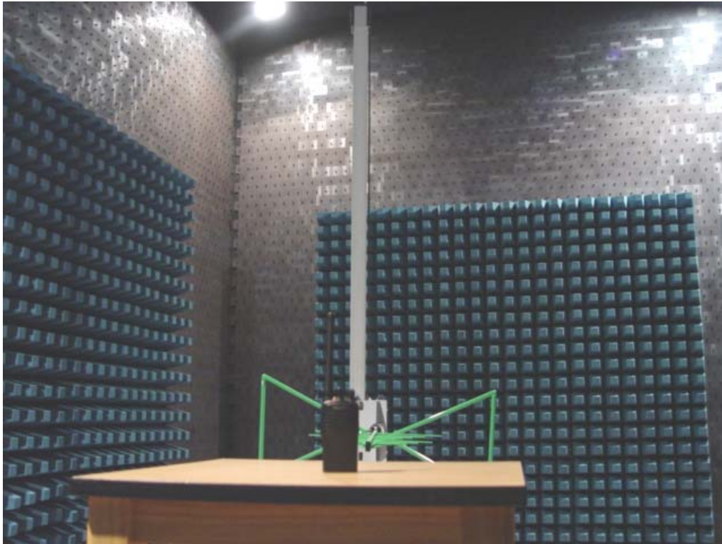
Photo 2 Radiated Emission Test
