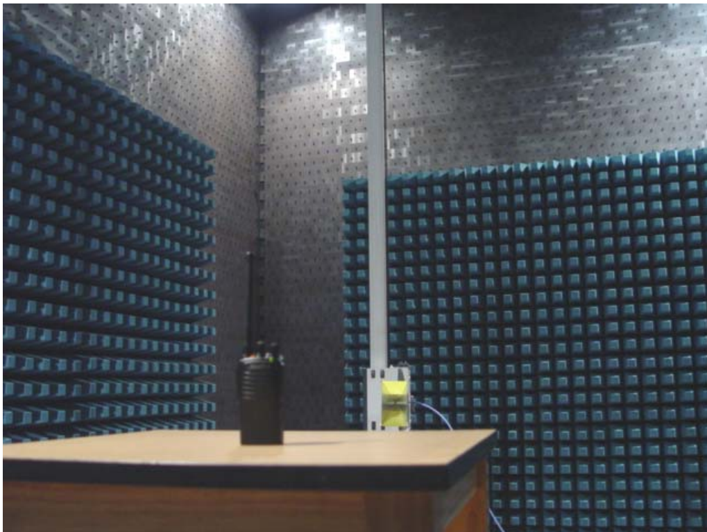
Photo 2 Radiated Emission Test
