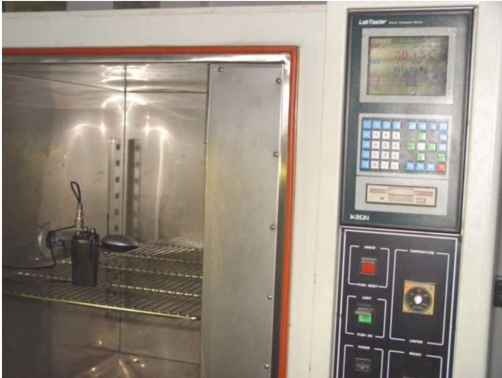
Photo 4 Transient frequency behavior Test
